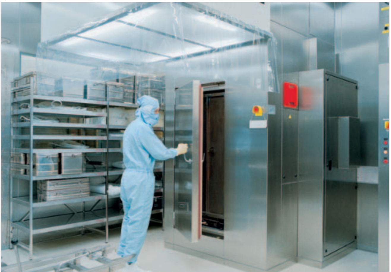
Dry heat steriliser VHSF-K1 with optional cooling chamber (two chamber system) for depyrogenation
